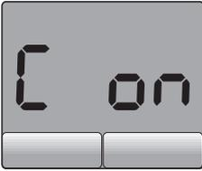
The same symbol will also be displayed whenever any button is pressed while the machine is child-locked.
