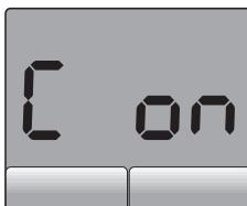
The same symbol will also be displayed whenever any button is pressed while the machine is child-locked.
