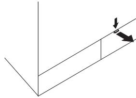
If it is composed of one piece, hold it from both sides and open it by pulling out.
